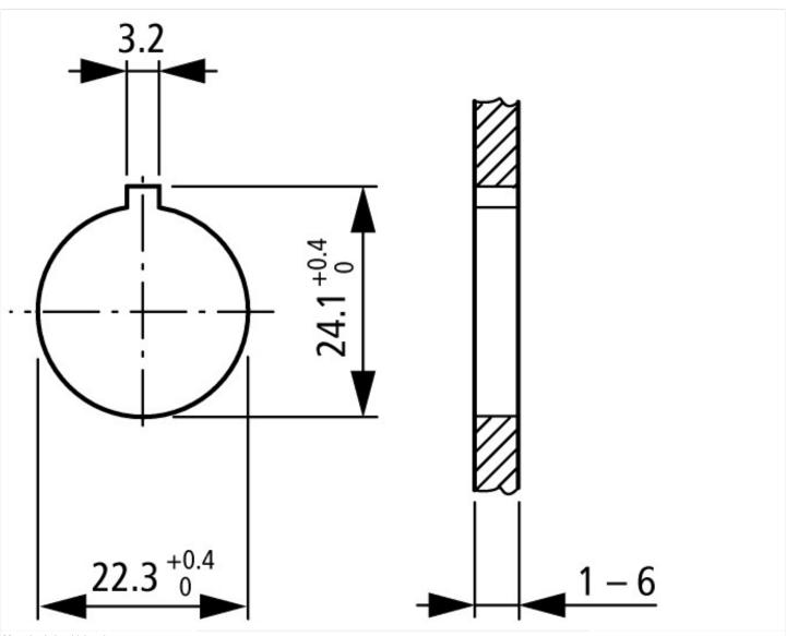
Mounting hole with lug slot
