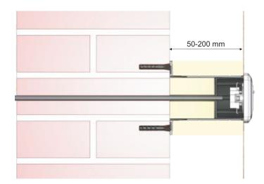
There is necessary to cut the carrier including inserted insulation before installation depending on layer thickness insulation.
