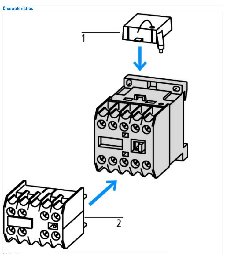
1: Suppressor 2: Auxiliary contact module
